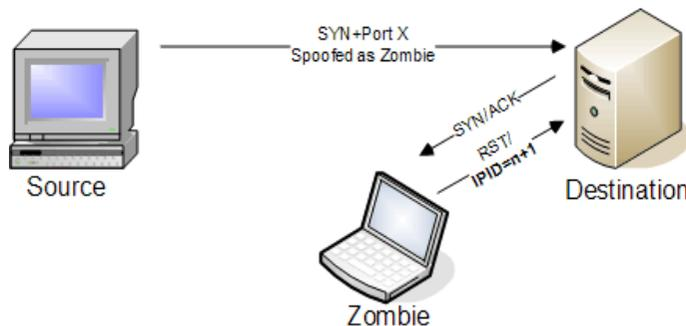
Step 3: Nmap repeats the original SYN/ACK probe of the zombie station. If the IPID has incremented, then the port that was spoofed in the original SYN frame is open on the destination device.
